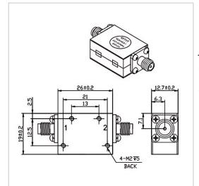
RF Solution offer a wide selection of Dual Junction Isolator for global customers. TG2619CS is a Dual Junction Isolator in Frequency Range of 8.0~12.0 GHz. It is made of high quality materials under a high standard, the Bandwidth Max of this product is 100%, Insertion Loss Max is 0.60~1.20 dB and Isolation Min is 32.0~50.0 dB. The component has a good working performance and stability, it is ideal for handling a Forward Power of 30 W.
