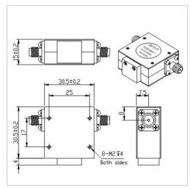
RF Solution offer a wide selection of Coaxial Isolator for global customers. TG3030BS is a Coaxial Isolator in Frequency Range of 2.0~6.0 GHz. It is made of high quality materials under a high standard, the Bandwidth Max of this product is 100%, Insertion Loss Max is 0.85~1.70 dB and Isolation Min is 12.0 dB. The component has a good working performance and stability, it is ideal for handling a Forward Power of 50 W.
