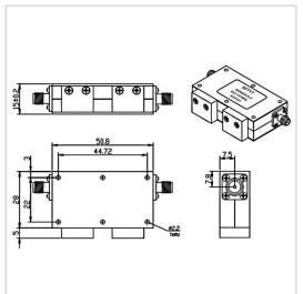
RF Solution offer a wide selection of Dual Junction Isolator for global customers. TG4223BS is a Dual Junction Isolator in Frequency Range of 4.0~8.0 GHz. It is made of high quality materials under a high standard, the Bandwidth Max of this product is 100%, Insertion Loss Max is 0.80~1.00 dB and Isolation Min is 36.0~40.0 dB. The component has a good working performance and stability, it is ideal for handling a Forward Power of 50 W.
