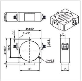
RF Solution offer a wide selection of Coaxial Isolator for global customers. TG4550XS is a Coaxial Isolator in Frequency Range of 250~1400 MHz. It is made of high quality materials under a high standard, the Bandwidth Max of this product is 40%, Insertion Loss Max is 0.25~0.80 dB and Isolation Min is 18.0~23.0 dB. The component has a good working performance and stability, it is ideal for handling a Forward Power of 100 W.
