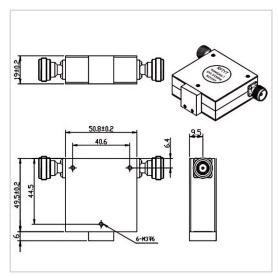
RF Solution offer a wide selection of Coaxial Isolator for global customers. TG5050AN is a Coaxial Isolator in Frequency Range of 1.25~3.0 MHz. It is made of high quality materials under a high standard, the Bandwidth Max of this product is 100%, Insertion Loss Max is 0.50~0.80 dB and Isolation Min is 16.0~18.0 dB. The component has a good working performance and stability, it is ideal for handling a Forward Power of 150 W.
