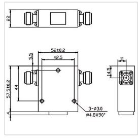
RF Solution offer a wide selection of Coaxial Isolator for global customers. TG5258EN is a Coaxial Isolator in Frequency Range of 150~330 MHz. It is made of high quality materials under a high standard, the Bandwidth Max of this product is 20%, Insertion Loss Max is 0.30~0.90 dB and Isolation Min is 18.0~23.0 dB. The component has a good working performance and stability, it is ideal for handling a Forward Power of 300 W.
