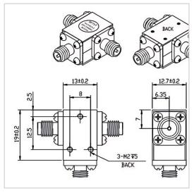
RF Solution offer a wide selection of Coaxial Circulator for global customers. TH1319CS is a Coaxial Circulator in Frequency Range of  $6.0\sim12.0$  GHz. It is made of high quality materials under a high standard, the Bandwidth Max of this product is 100%, Insertion Loss Max is  $0.40\sim0.60$  dB and Isolation Min is  $16.0\sim23.0$  dB. The component has a good working performance and stability, it is ideal for handling a Power of 30 W.
