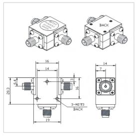
RF Solution offer a wide selection of Coaxial Circulator for global customers. TH1620BS is a Coaxial Circulator in Frequency Range of 6.0~18.0 GHz. It is made of high quality materials under a high standard, the Bandwidth Max of this product is 100%, Insertion Loss Max is 0.60~1.50 dB and Isolation Min is 12.0~18.0 dB. The component has a good working performance and stability, it is ideal for handling a Power of 30 W.
