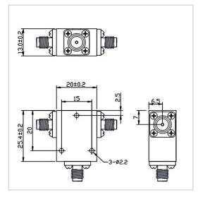
RF Solution offer a wide selection of Coaxial Circulator for global customers. TH2025XS is a Coaxial Circulator in Frequency Range of 1700~5000 MHz. It is made of high quality materials under a high standard, the Bandwidth Max of this product is 20%, Insertion Loss Max is 0.25~0.50 dB and Isolation Min is 18.0~25.0 dB. The component has a good working performance and stability, it is ideal for handling a Forward Power of 100 W.
