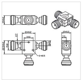
RF Solution offer a wide selection of Coaxial Circulator for global customers. TH2123BN is a Coaxial Circulator in Frequency Range of 4.0~8.0 GHz. It is made of high quality materials under a high standard, the Bandwidth Max of this product is 100%, Insertion Loss Max is 0.40~0.60 dB and Isolation Min is 18.0~20.0 dB. The component has a good working performance and stability, it is ideal for handling a Power of 100 W.
