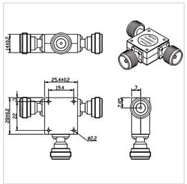
RF Solution offer a wide selection of Coaxial Circulator for global customers. TH2528CN is a Coaxial Circulator in Frequency Range of 3.0~6.0 GHz. It is made of high quality materials under a high standard, the Bandwidth Max of this product is 100%, Insertion Loss Max is 0.40~0.50 dB and Isolation Min is 18.0~20.0 dB. The component has a good working performance and stability, it is ideal for handling a Power of 150 W.
