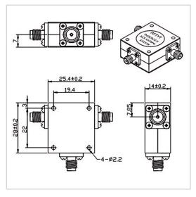
RF Solution offer a wide selection of Coaxial Circulator for global customers. TH2528CS is a Coaxial Circulator in Frequency Range of  $3.0\sim6.0$  GHz. It is made of high quality materials under a high standard, the Bandwidth Max of this product is 100%, Insertion Loss Max is  $0.40\sim0.50$  dB and Isolation Min is  $18.0\sim20.0$  dB. The component has a good working performance and stability, it is ideal for handling a Power of 100 W.
