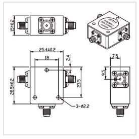
RF Solution offer a wide selection of Coaxial Circulator for global customers. TH2528XS is a Coaxial Circulator in Frequency Range of  $700\sim5000$  MHz. It is made of high quality materials under a high standard, the Bandwidth Max of this product is 25%, Insertion Loss Max is  $0.30\sim0.60$  dB and Isolation Min is  $16.0\sim25.0$  dB. The component has a good working performance and stability, it is ideal for handling a Forward Power of 100 W.
