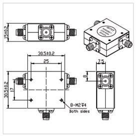
RF Solution offer a wide selection of Coaxial Circulator for global customers. TH3030BS is a Coaxial Circulator in Frequency Range of  $2.0\sim6.0$  GHz. It is made of high quality materials under a high standard, the Bandwidth Max of this product is 100%, Insertion Loss Max is  $0.85\sim1.70$  dB and Isolation Min is 12.0 dB. The component has a good working performance and stability, it is ideal for handling a Forward Power of 50 W.
