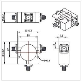
RF Solution offer a wide selection of Coaxial Circulator for global customers. TH3232XS is a Coaxial Circulator in Frequency Range of 700~3000 MHz. It is made of high quality materials under a high standard, the Bandwidth Max of this product is 25%, Insertion Loss Max is 0.30~0.60 dB and Isolation Min is 18.0~23.0 dB. The component has a good working performance and stability, it is ideal for handling a Forward Power of 100 W.
