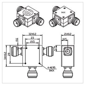
RF Solution offer a wide selection of Coaxial Circulator for global customers. TH3234AN is a Coaxial Circulator in Frequency Range of 2.0~4.0 GHz. It is made of high quality materials under a high standard, the Bandwidth Max of this product is 100%, Insertion Loss Max is 0.40~0.50 dB and Isolation Min is 18.0~20.0 dB. The component has a good working performance and stability, it is ideal for handling a Forward Power of 150 W.
