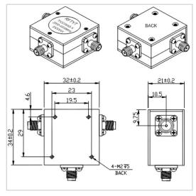
RF Solution offer a wide selection of Coaxial Circulator for global customers. TH3234AS is a Coaxial Circulator in Frequency Range of 2.0~4.0 GHz. It is made of high quality materials under a high standard, the Bandwidth Max of this product is 100%, Insertion Loss Max is 0.40~0.50 dB and Isolation Min is 18.0~20.0 dB. The component has a good working performance and stability, it is ideal for handling a Forward Power of 100 W.
