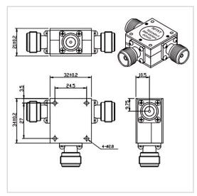
RF Solution offer a wide selection of Coaxial Circulator for global customers. TH3234BN is a Coaxial Circulator in Frequency Range of 2.0~4.0 GHz. It is made of high quality materials under a high standard, the Bandwidth Max of this product is 100%, Insertion Loss Max is 0.40~0.50 dB and Isolation Min is 18.0~20.0 dB. The component has a good working performance and stability, it is ideal for handling a Forward Power of 150 W.
