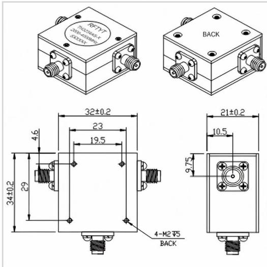
RF Solution offer a wide selection of Coaxial Circulator for global customers. TH3234BS is a Coaxial Circulator in Frequency Range of 2.0~4.0 GHz. It is made of high quality materials under a high standard, the Bandwidth Max of this product is 100%, Insertion Loss Max is 0.40~0.50 dB and Isolation Min is 18.0~20.0 dB. The component has a good working performance and stability, it is ideal for handling a Forward Power of 100 W.
