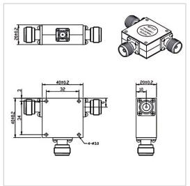
RF Solution offer a wide selection of Coaxial Circulator for global customers. TH4040AN is a Coaxial Circulator in Frequency Range of 1.25~3.0 GHz. It is made of high quality materials under a high standard, the Bandwidth Max of this product is 100%, Insertion Loss Max is 0.50~0.60 dB and Isolation Min is 17.0~18.0 dB. The component has a good working performance and stability, it is ideal for handling a Forward Power of 100 W.
