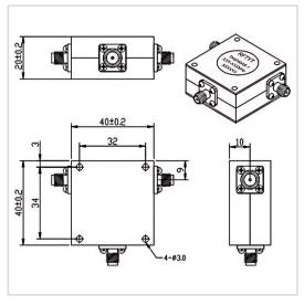
RF Solution offer a wide selection of Coaxial Circulator for global customers. TH4040AS is a Coaxial Circulator in Frequency Range of 1.25~3.0 GHz. It is made of high quality materials under a high standard, the Bandwidth Max of this product is 100%, Insertion Loss Max is 0.50~0.60 dB and Isolation Min is 17.0~18.0 dB. The component has a good working performance and stability, it is ideal for handling a Forward Power of 100 W.
