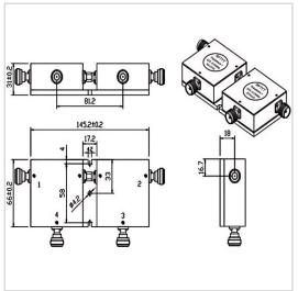
RF Solution offer a wide selection of Dual Junction Circulator for global customers. THH14566KN is a Dual Junction Circulator in Frequency Range of 1.0-2.0GHz. It is made of high quality materials under a high standard, the Bandwidth Max of this product is Full, Insertion Loss Max is 1.4 dB and Isolation Min is 32.0 dB. The component has a good working performance and stability, it is ideal for handling a Forward Power of 100 W.
