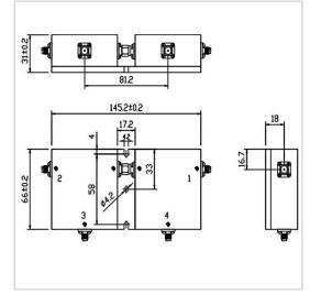
RF Solution offer a wide selection of Dual Junction Circulator for global customers. THH14566KS is a Dual Junction Circulator in Frequency Range of 1.0-2.0GHz. It is made of high quality materials under a high standard, the Bandwidth Max of this product is Full, Insertion Loss Max is 1.3 dB and Isolation Min is 34.0 dB. The component has a good working performance and stability, it is ideal for handling a Forward Power of 100 W.
