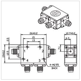
RF Solution offer a wide selection of Dual Junction Circulator for global customers. THH2619CS is a Dual Junction Circulator in Frequency Range of 8.0-12.0GHz. It is made of high quality materials under a high standard, the Bandwidth Max of this product is Full, Insertion Loss Max is 1.0 dB and Isolation Min is 36.0 dB. The component has a good working performance and stability, it is ideal for handling a Forward Power of 30 W.
