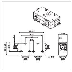
RF Solution offer a wide selection of Dual Junction Circulator for global customers. THH4223BS is a Dual Junction Circulator in Frequency Range of 4.0-8.0GHz. It is made of high quality materials under a high standard, the Bandwidth Max of this product is Full, Insertion Loss Max is 1.2 dB and Isolation Min is 34.0 dB. The component has a good working performance and stability, it is ideal for handling a Forward Power of 50 W.
