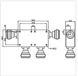
RF Solution offer a wide selection of Dual Junction Circulator for global customers. THH5028CN is a Dual Junction Circulator in Frequency Range 3.0-6.0GHz. It is made of high quality materials under a high standard, the Bandwidth Max of this product is Full, Insertion Loss Max is 1.0 dB and Isolation Min is 36.0 dB. The component has a good working performance and stability, it is ideal for handling a Forward Power of 100 W.
