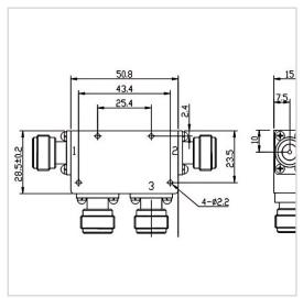
RF Solution offer a wide selection of Dual Junction Circulator for global customers. THH5028XN is a Dual Junction Circulator in Frequency Range of 700~5000 MHz. It is made of high quality materials under a high standard, the Bandwidth Max of this product is 20%, Insertion Loss Max is 1.2 dB and Isolation Min is 34 dB. The component has a good working performance and stability, it is ideal for handling a Forward Power of 200 W.
