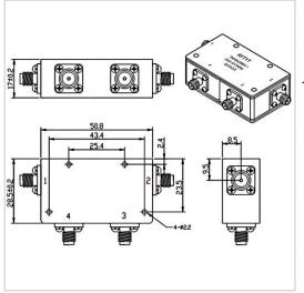
RF Solution offer a wide selection of Dual Junction Circulator for global customers. THH5028XS is a Dual Junction Circulator in Frequency Range of 700~4200 MHz. It is made of high quality materials under a high standard, the Bandwidth Max of this product is 20%, Insertion Loss Max is 1.2 dB and Isolation Min is 34 dB. The component has a good working performance and stability, it is ideal for handling a Forward Power of 100 W.
