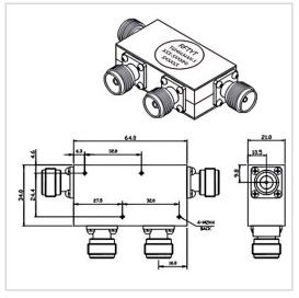
RF Solution offer a wide selection of Dual Junction Circulator for global customers. THH6434AN is a Dual Circulator in Frequency lunction Range 2.0-4.0GHz. It is made of high quality materials under a high standard, the Bandwidth Max of this product is Full, Insertion Loss Max is 1.2 dB and Isolation Min is 36.0 dB. The component has a good working performance and stability, it is ideal for handling a Forward Power of 100 W.
