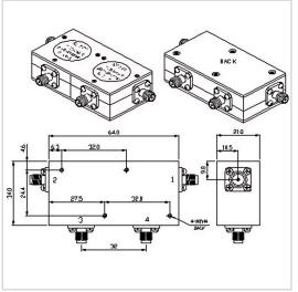
RF Solution offer a wide selection of Dual Junction Circulator for global customers. THH6434AS is a Dual Junction Circulator in Frequency Range of 2.0-4.0GHz. It is made of high quality materials under a high standard, the Bandwidth Max of this product is Full, Insertion Loss Max is 1.2 dB and Isolation Min is 36.0 dB. The component has a good working performance and stability, it is ideal for handling a Forward Power of 100 W.
