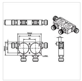
RF Solution offer a wide selection of Dual Junction Circulator for global customers. THH7038XN is a Dual Junction Circulator in Frequency Range of 400-1850 MHz. It is made of high quality materials under a high standard, the Bandwidth Max of this product is 20%, Insertion Loss Max is 1.2 dB and Isolation Min is 36.0 dB. The component has a good working performance and stability, it is ideal for handling a Forward Power of 300 W.
