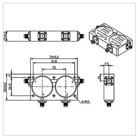
RF Solution offer a wide selection of Dual Junction Circulator for global customers. THH7038XS is a Dual Junction Circulator in Frequency Range of 400-1850 MHz. It is made of high quality materials under a high standard, the Bandwidth Max of this product is 20%, Insertion Loss Max is 1.2 dB and Isolation Min is 36.0 dB. The component has a good working performance and stability, it is ideal for handling a Forward Power of 100 W.
