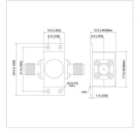
RF Solution offer a wide selection of Coaxial Isolator for global customers. UIYBCI1025A is a Coaxial Isolator in Frequency Range of 18.0~28.0 GHz. It is made of high quality materials under a high standard, the Bandwidth Max of this product is 100%, Insertion Loss Max is 0.70~0.90 dB and Isolation Min is 20.0 dB. The component has a good working performance and stability, it is ideal for handling a Forward Power of 10 W.
