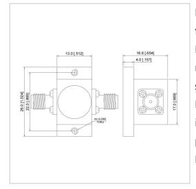
RF Solution offer a wide selection of Coaxial Isolator for global customers. UIYBCI1326B is a Coaxial Isolator in Frequency Range of 22.0~33.0 GHz. It is made of high quality materials under a high standard, the Bandwidth Max of this product is 100%, Insertion Loss Max is 1.30~1.60 dB and Isolation Min is 15.0~16.0 dB. The component has a good working performance and stability, it is ideal for handling a Forward Power of 10 W.
