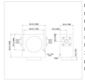
RF Solution offer a wide selection of Broadband Isolator for global customers. UIYBCI3232A is a Broadband Isolator in Frequency Range of 960~1215 MHz. It is made of high quality materials under a high standard, the Bandwidth Max of this product is 100%, Insertion Loss Max is 0.40 dB and Isolation Min is 20.0 dB. The component has a good working performance and stability, it is ideal for handling a Forward Power of 100/200 W.
