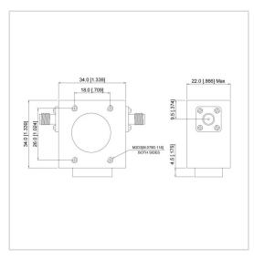
RF Solution offer a wide selection of Broadband Isolator for global customers. UIYBCI3434B is a Broadband Isolator in Frequency Range of 700~900 MHz. It is made of high quality materials under a high standard, the Bandwidth Max of this product is 100%, Insertion Loss Max is 0.40 dB and Isolation Min is 18.0 dB. The component has a good working performance and stability, it is ideal for handling a Forward Power of 100/200 W.
