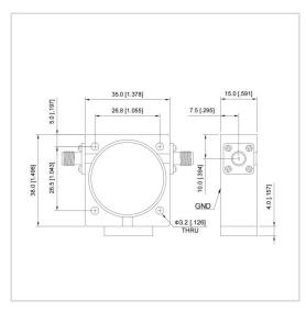
RF Solution offer a wide selection of Broadband Isolator for global customers. UIYBCI3538C is a Broadband Isolator in Frequency Range of 600~800 MHz. It is made of high quality materials under a high standard, the Bandwidth Max of this product is 100%, Insertion Loss Max is 0.50 dB and Isolation Min is 18.0 dB. The component has a good working performance and stability, it is ideal for handling a Forward Power of 300/100 W.
