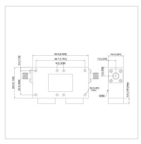
RF Solution offer a wide selection of Dual Junction Isolator for global customers. UIYBCI5028A is a Dual Junction Isolator in Frequency Range of 3.0~6.0 GHz. It is made of high quality materials under a high standard, the Bandwidth Max of this product is 100%, Insertion Loss Max is 1.00 dB and Isolation Min is 36.0 dB. The component has a good working performance and stability, it is ideal for handling a Forward Power of 100 W.
