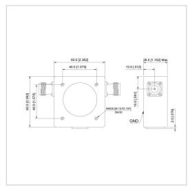
RF Solution offer a wide selection of Broadband Isolator for global customers. UIYBCI6060A is a Broadband Isolator in Frequency Range of 66~88 MHz. It is made of high quality materials under a high standard, the Bandwidth Max of this product is 100%, Insertion Loss Max is 1.30 dB and Isolation Min is 18.0 dB. The component has a good working performance and stability, it is ideal for handling a Forward Power of 100 W.
