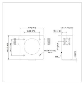
RF Solution offer a wide selection of Broadband Isolator for global customers. UIYBCI6060D is a Broadband Isolator in Frequency Range of 136~174 MHz. It is made of high quality materials under a high standard, the Bandwidth Max of this product is 100%, Insertion Loss Max is 0.65 dB and Isolation Min is 20.0 dB. The component has a good working performance and stability, it is ideal for handling a Forward Power of 100 W.
