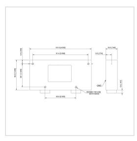
RF Solution offer a wide selection of Dual Junction Isolator for global customers. UIYBDI10149A is a Dual Junction Isolator in Frequency Range of 1.35~2.7 GHz. It is made of high quality materials under a high standard, the Bandwidth Max of this product is 100%, Insertion Loss Max is 1.00 dB and Isolation Min is 36.0 dB. The component has a good working performance and stability, it is ideal for handling a Forward Power of 100 W.
