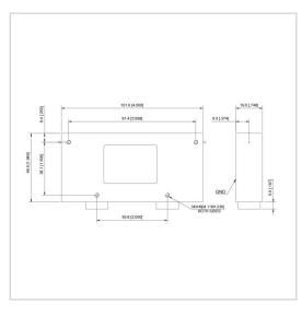
RF Solution offer a wide selection of Dual Junction Isolator for global customers. UIYBDI10149B is a Dual Junction Isolator in Frequency Range of 1.5~3.0 GHz. It is made of high quality materials under a high standard, the Bandwidth Max of this product is 100%, Insertion Loss Max is 1.00 dB and Isolation Min is 34.0 dB. The component has a good working performance and stability, it is ideal for handling a Forward Power of 100 W.
