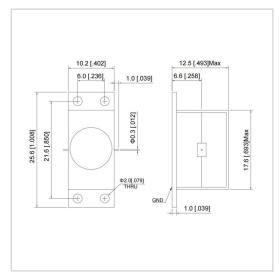
RF Solution offer a wide selection of Drop in Isolator for global customers. UIYBDI1025A is a Drop in Isolator in Frequency Range of 18.0~28.0 GHz. It is made of high quality materials under a high standard, the Bandwidth Max of this product is 100%, Insertion Loss Max is 0.70~0.90 dB and Isolation Min is 20.0 dB. The component has a good working performance and stability, it is ideal for handling a Forward Power of 10 W.
