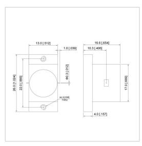
RF Solution offer a wide selection of Drop in Isolator for global customers. UIYBDI1326A is a Drop in Isolator in Frequency Range of 26.5~40.0 GHz. It is made of high quality materials under a high standard, the Bandwidth Max of this product is 100%, Insertion Loss Max is 1.50~1.70 dB and Isolation Min is 12.0~14.0 dB. The component has a good working performance and stability, it is ideal for handling a Forward Power of 10 W.
