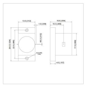
RF Solution offer a wide selection of Drop in Isolator for global customers. UIYBDI1326B is a Drop in Isolator in Frequency Range of 22.0~33.0 GHz. It is made of high quality materials under a high standard, the Bandwidth Max of this product is 100%, Insertion Loss Max is 1.30~1.60 dB and Isolation Min is 15.0~16.0 dB. The component has a good working performance and stability, it is ideal for handling a Forward Power of 10 W.
