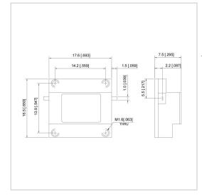
RF Solution offer a wide selection of Dual Junction Isolator for global customers. UIYBDI1716A is a Dual Junction Isolator in Frequency Range of 8.0~12.0 GHz. It is made of high quality materials under a high standard, the Bandwidth Max of this product is 100%, Insertion Loss Max is 1.00 dB and Isolation Min is 36.0 dB. The component has a good working performance and stability, it is ideal for handling a Forward Power of 30 W.
