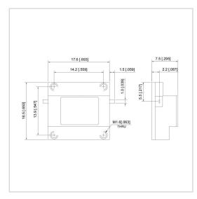
RF Solution offer a wide selection of Dual Junction Isolator for global customers. UIYBDI1716B is a Dual Junction Isolator in Frequency Range of 12.0~18.0 GHz. It is made of high quality materials under a high standard, the Bandwidth Max of this product is 100%, Insertion Loss Max is 1.20 dB and Isolation Min is 36.0 dB. The component has a good working performance and stability, it is ideal for handling a Forward Power of 30 W.
