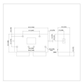
RF Solution offer a wide selection of Dual Junction Isolator for global customers. UIYBDI4222A is a Dual Junction Isolator in Frequency Range of 4.0~8.0 GHz. It is made of high quality materials under a high standard, the Bandwidth Max of this product is 100%, Insertion Loss Max is 1.00 dB and Isolation Min is 36.0 dB. The component has a good working performance and stability, it is ideal for handling a Forward Power of 100 W.
