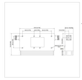
RF Solution offer a wide selection of Dual Junction Isolator for global customers. UIYCDI12075A is a Dual Junction Isolator in Frequency Range of 45~270 MHz. It is made of high quality materials under a high standard, the Bandwidth Max of this product is 40%, Insertion Loss Max is 1.00~3.60 dB and Isolation Min is 36.0~45.0 dB. The component has a good working performance and stability, it is ideal for handling a Forward Power of 100/150/200 W.
