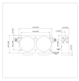
RF Solution offer a wide selection of Dual Junction Isolator for global customers. UIYCDI7038A is a Dual Junction Isolator in Frequency Range of  $200\sim1875$  MHz. It is made of high quality materials under a high standard, the Bandwidth Max of this product is 30%, Insertion Loss Max is  $0.60\sim1.30$  dB and Isolation Min is  $30.0\sim60.0$  dB. The component has a good working performance and stability, it is ideal for handling a Forward Power of 100/300 W.
